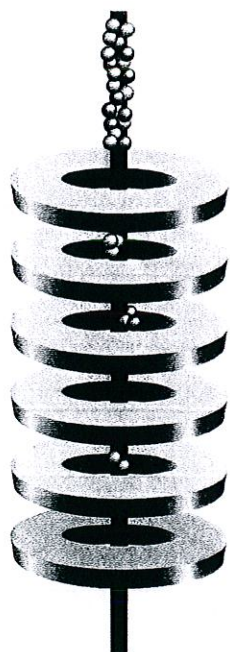
Figure 13: Once released into the T-wave region, a traveling waveform drives the ions through a neutral buffer gas (typically Nitrogen at 0.5 mbar) separating them by their mobility.
