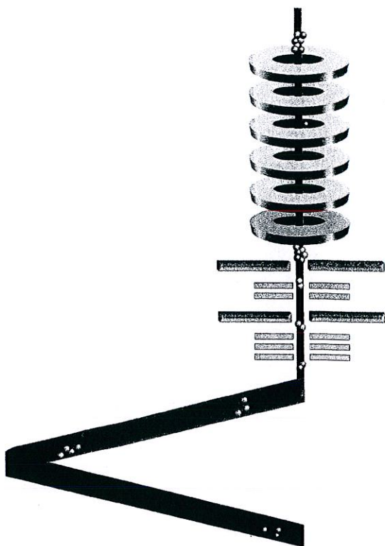
Figure 14: The separated 'packets' of ions with the same mobility characteristics are then passed to the TOF drift tube where their m/z values are measured. The system, therefore, has the potential to separate isobaric ions (ions of identical m/z ) or those of very similar m/z prior to mass analysis increasing the overall peak capacity of the MS or LC/MS system.
